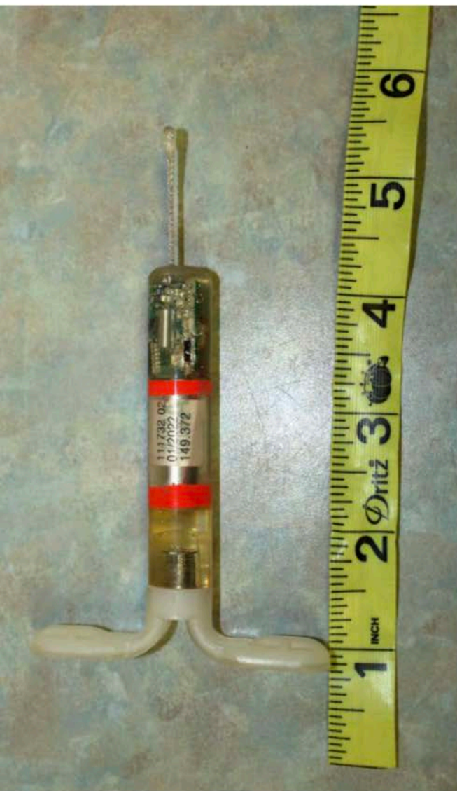
A Vaginal Implant Transmitter (VIT), often deployed in pregnant, wild deer to track birth events for fawn survival studies. We used modified VITs that recorded the internal temperature of deer to identify the physiological cost of pregnancy and high temperatures.
